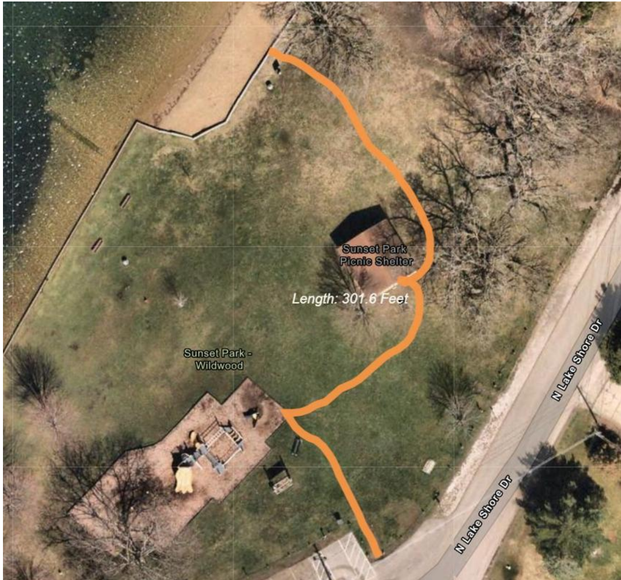
General overview of a new ADA accessible paved path at Sunset Beach Park, 33270 N Lake Shore Drive, Wildwood, IL. Exact placement will be determined by using the best practices with consideration of access points to key elements and grades of the area, causing the least disturbance to existing trees. The length is approximately 300 feet.
